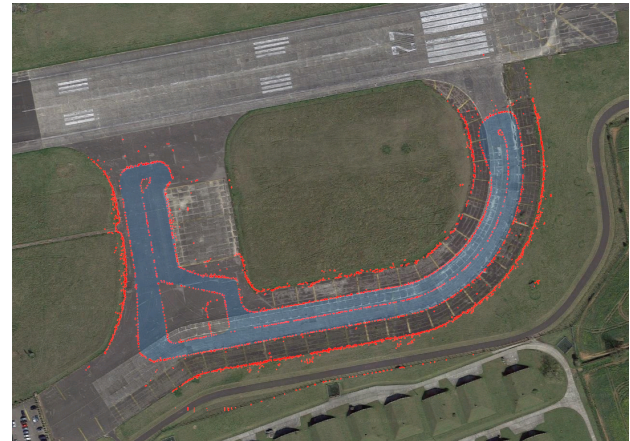
Figure 7. Areal footage of the test field with overlaid LIDAR scans (red) visualizing the test track (blue) framed by cones.
