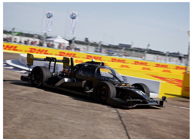
Figure 1. DevBot - The development vehicle of Roborace holding various sensors and control units.[1]
