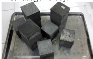
Fig. 3. The test cubic specimens of 70.7 \times 70.7 \times 70.7 mm.
