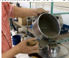
Fig. 2. Determination of the slump-flow of concrete mixture.
