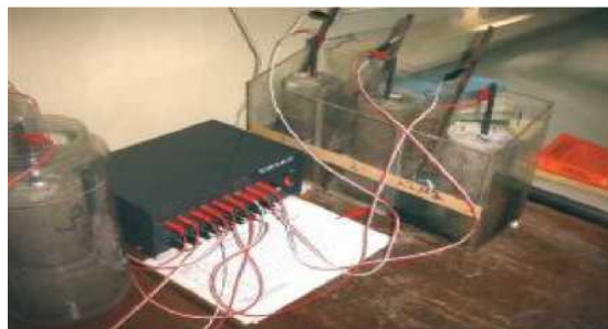
Fig. 6. Samples of concrete, prepared for testing and measuring of amperage through concrete experimental sample.
