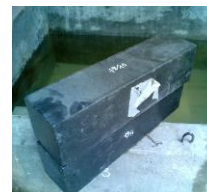
Fig. 4. The test prismatic specimens of fine-grained concrete.
