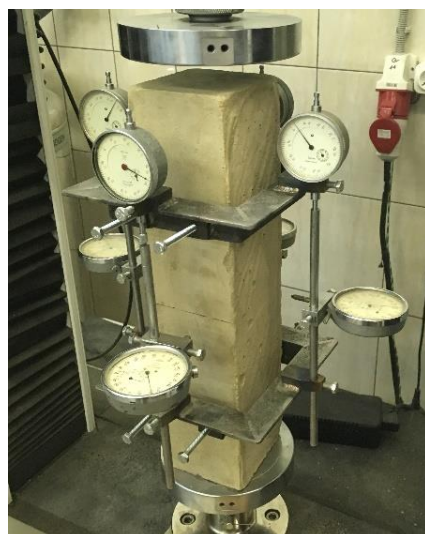
Fig. 6. Definition of elasticity modulus of stone-concrete.
