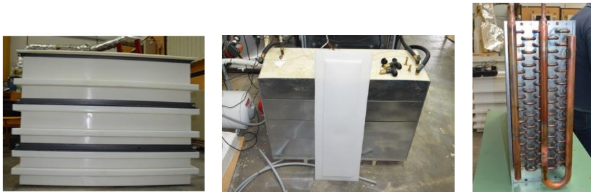
Fig. 1. (a) The HTES tank without and with insulation (b) View of the HE.
