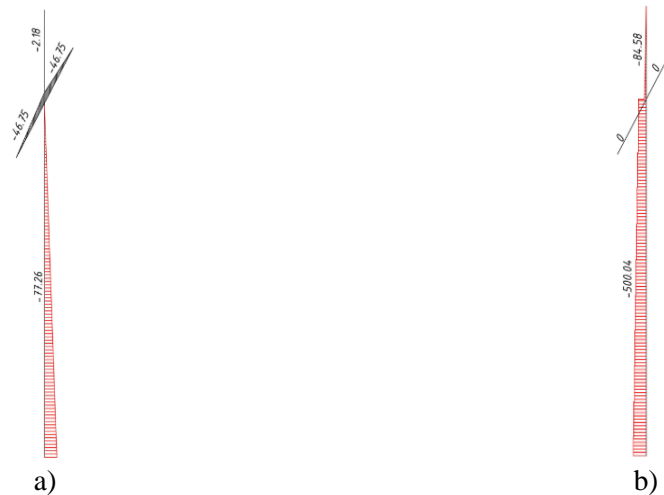
Fig. 5. Diagrams of bending moments without wires breakage (a – Maximum moment M_x , b – Maximum compressive stress N ).
