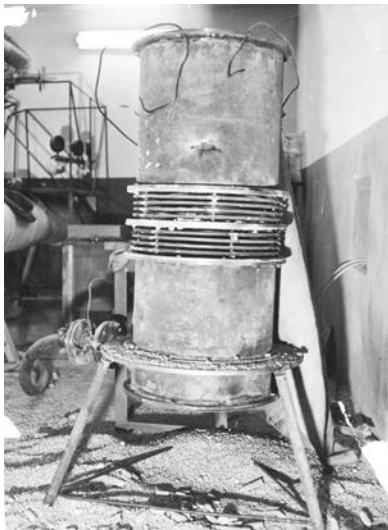
Fig. 3. Installation for threshing, a tube with a diameter of 500 mm.
