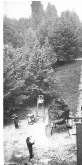
Fig. 4. The first test of an open vortex tube with a diameter of 1000 mm for threshing of corn cobs.
