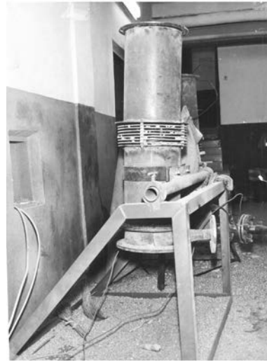
Fig. 2. Installation for threshing of corn cobs, a tube with a diameter of 300 mm.
