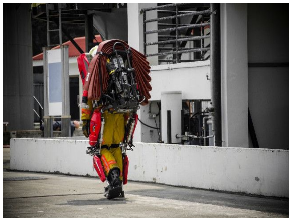
Fig. 2. Fire exoskeleton Auberon Pneumatic Exoskeleton, developed by the specialized car manufacturer Trigen Automotive in Singapore.
