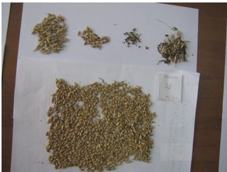
Fig. 2. A portion of bunker grain pile after having been segregated by fractions.
