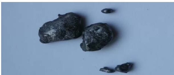
Fig. 4. Pig iron, obtained from reducing firing product
