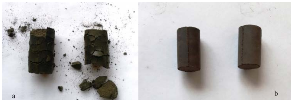
Fig. 1. General view of water-bonded briquettes (a) and strong briquettes with the special binder (b) in 24 hours after briquetting
