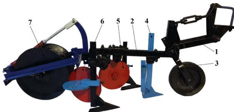
Fig. 1. The seeder gang: 1 - parallelogram mechanism; 2 - ridge; 3 - support wheel; 4 - coulters; 5, 6 - working bodies with right and left flat discs; 7 - roller-ridge former
