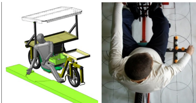
Fig. 2. Simulation of the picking process from the platform in the Compass 3D CAD system, and under laboratory conditions to study the reach zone during the assembly.
