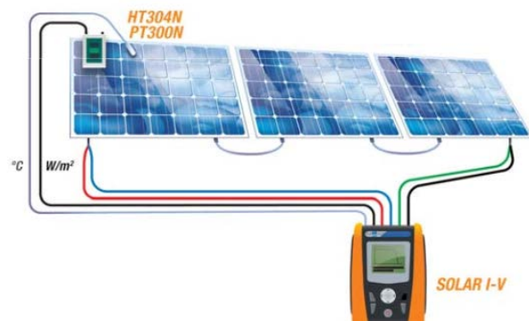
Fig. 8. Connection diagram of the device (I-V 400 model) to the solar module (DSM-240-C model).
