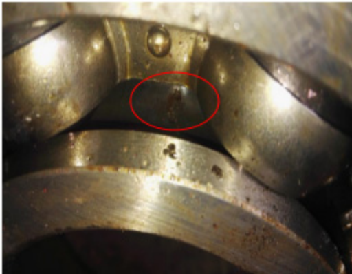
Figure 3: Large peeling, pits
