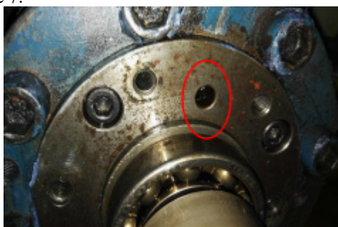
Figure 7 Machine seal return hole
