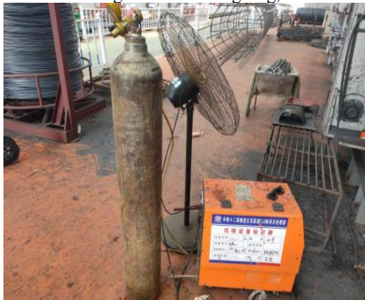
Figure 12. Rebar processing plant, prefabricated plant, tunnel steel structure using carbon dioxide protection welding
