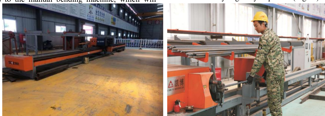
Figure 16. CNC bending of steel bars
