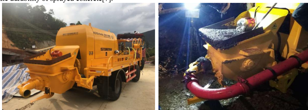
Figure 11. Tunnel wet sprayer
