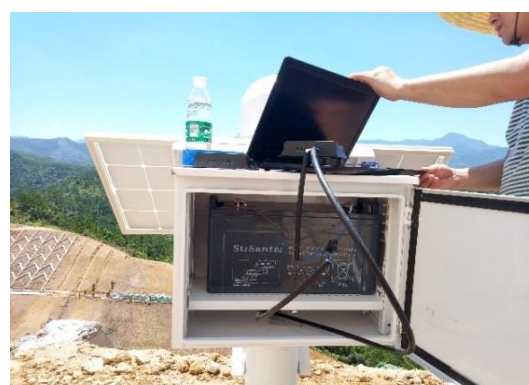
Figure 7. Automatic monitoring system for high slope deformation
