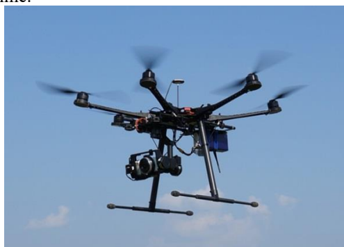
Figure 6. Automatic surface displacement monitoring equipment
