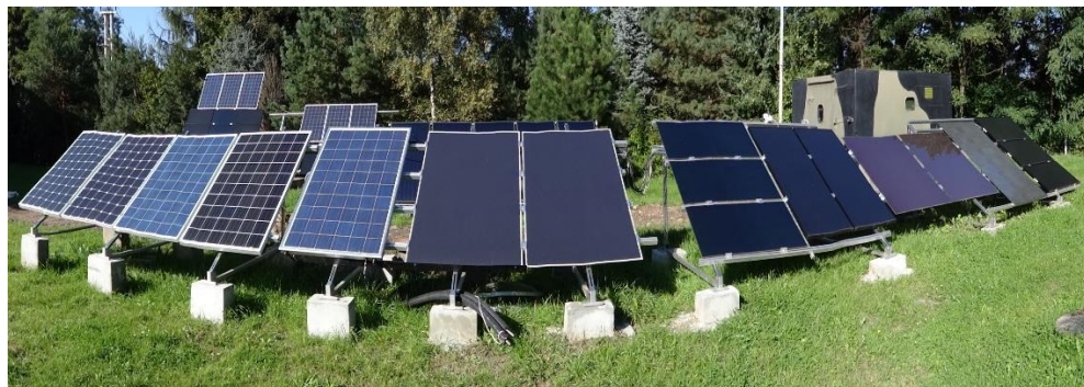
Fig. 1. The installation with different PV modules.
