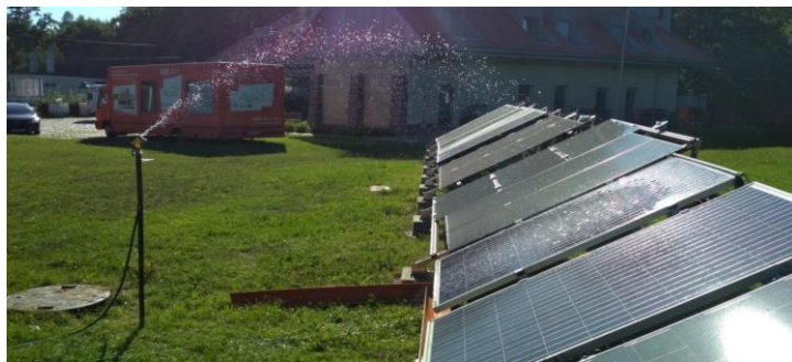
Fig. 2. Research stand with cooling by imitation of rain
