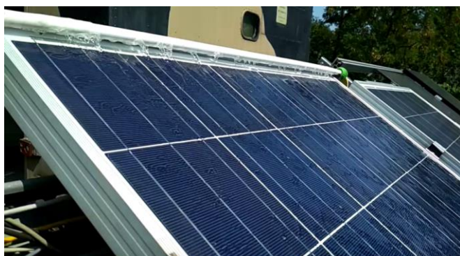
Fig. 3. Research stand with cooling by water film
