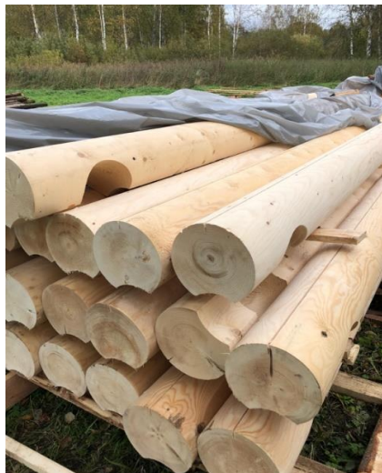
Fig. 13. Calibrated log for a new log house. The author of the photographs is Zhivotov D. A.
