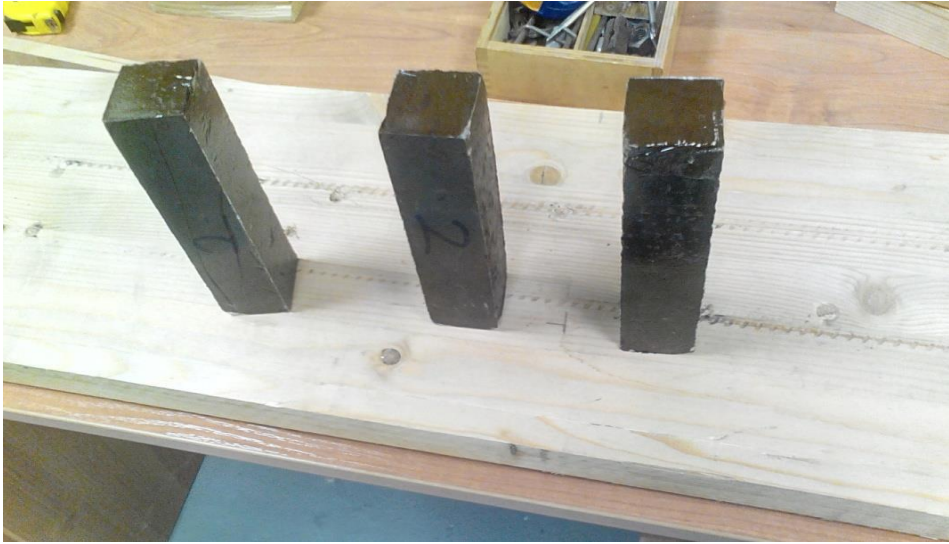
Fig. 6. Samples for obtaining the calculated characteristics of rubcon.
