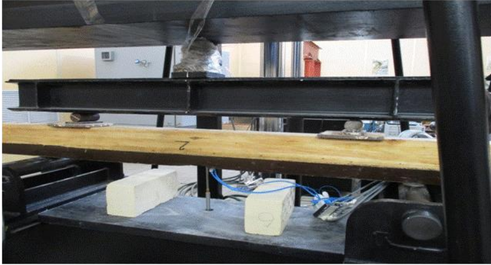
Fig. 8. Loading scheme of wood-rubcon reinforced composite bridge beams.
