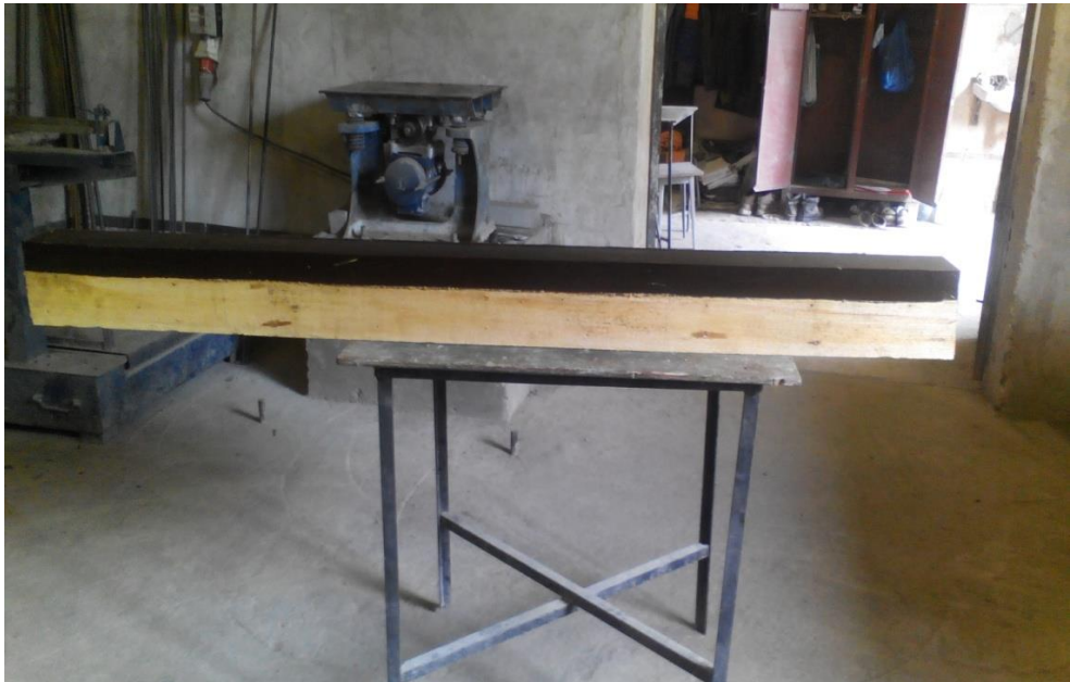
Fig. 5. General view of a wood-rubcon reinforced composite bridge beam.
