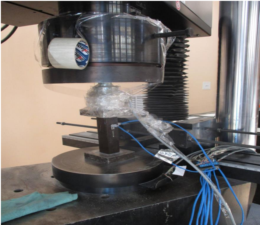
Fig. 11. Test pattern of rubcon concrete sample for deformation.
