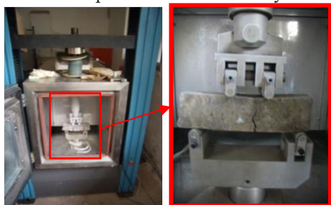
Fig.4 Bending test on artificial frozen soils
