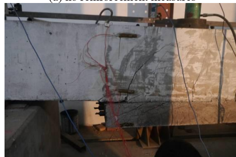
(b) reinforcement by enlarging section-prestress method
