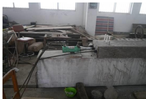
Fig.3 application of prestressing force
