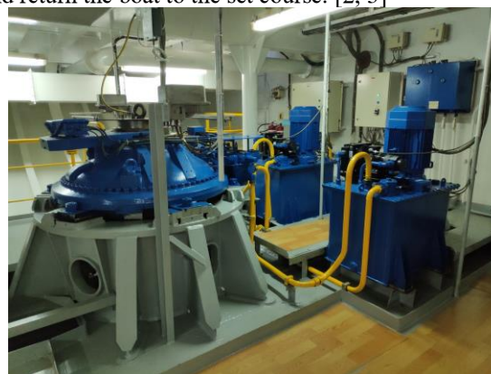
Fig. 1. Overview of steering gear hydraulic system
