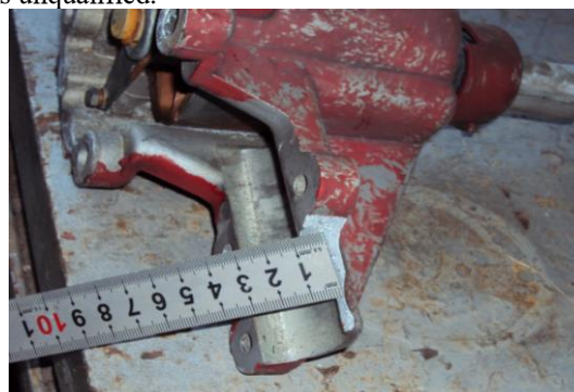
Fig. 7. Fracture morphology of the terminal block.
