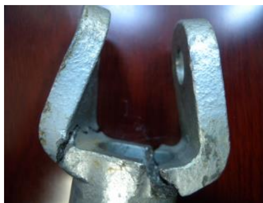
Fig. 4. Fracture morphology of the universal joint fork.
