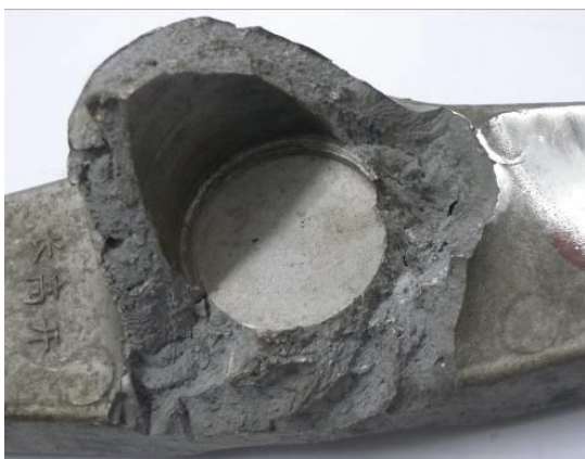
Fig. 1. Fracture morphology of the flange.
