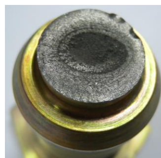
Fig. 6. Morphology of macro fracture of the bolt.
