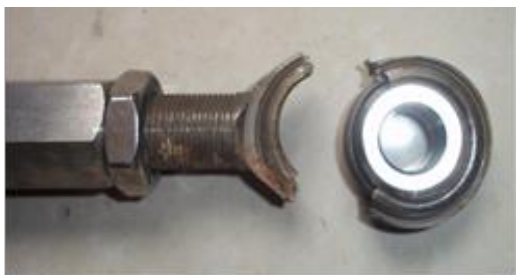
Fig. 5. The macroscopic feature of disconnected universal joint.
