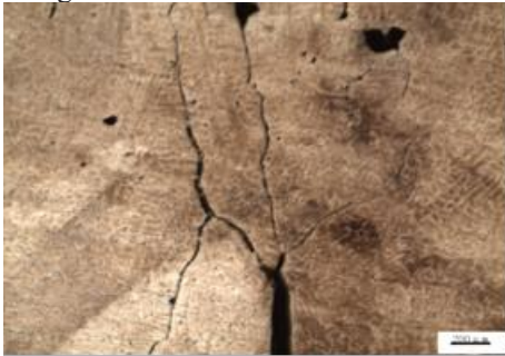
Fig.10. The picture of the intergranular crack in sample.
