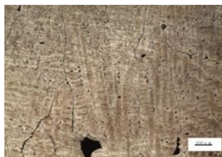
Fig.8. The picture of thick columnar crystal.
