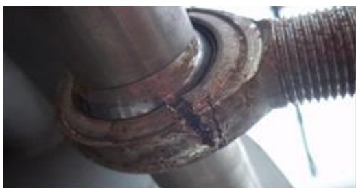
Fig. 6. The macroscopic feature of undisconnected universal joint.
