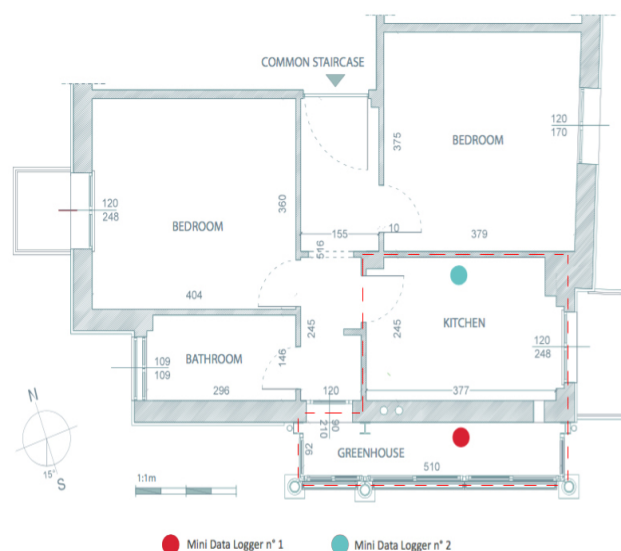
Fig. 3. Plan of the studied apartment with the position of the relevant recording thermometers.
