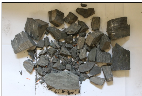
Fig. 2. The result of explosive loading of a ferrous quartzite slab
