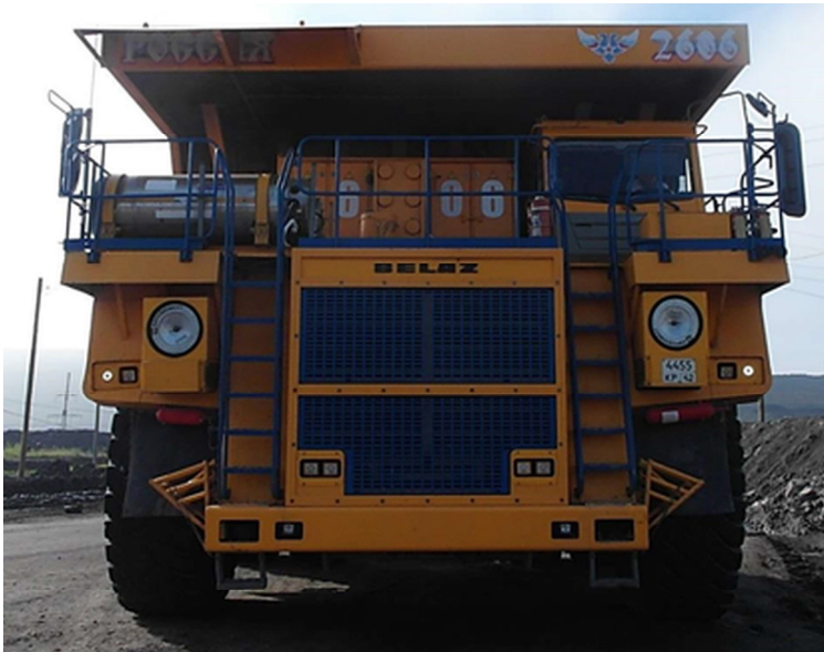
Fig. 1. The upgraded BelAZ-75131 dump truck using gas-diesel cycle.
