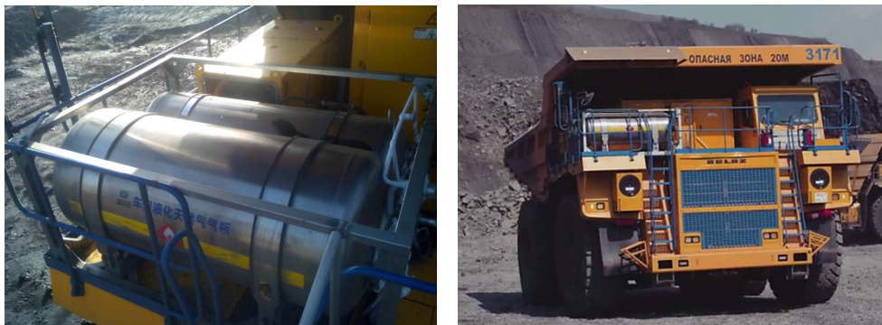
Fig. 7. Two horizontal cryogenic fuel tanks with volumes of 850 and 500 liters installed on the deck of the BelAZ 75131 dump truck.
