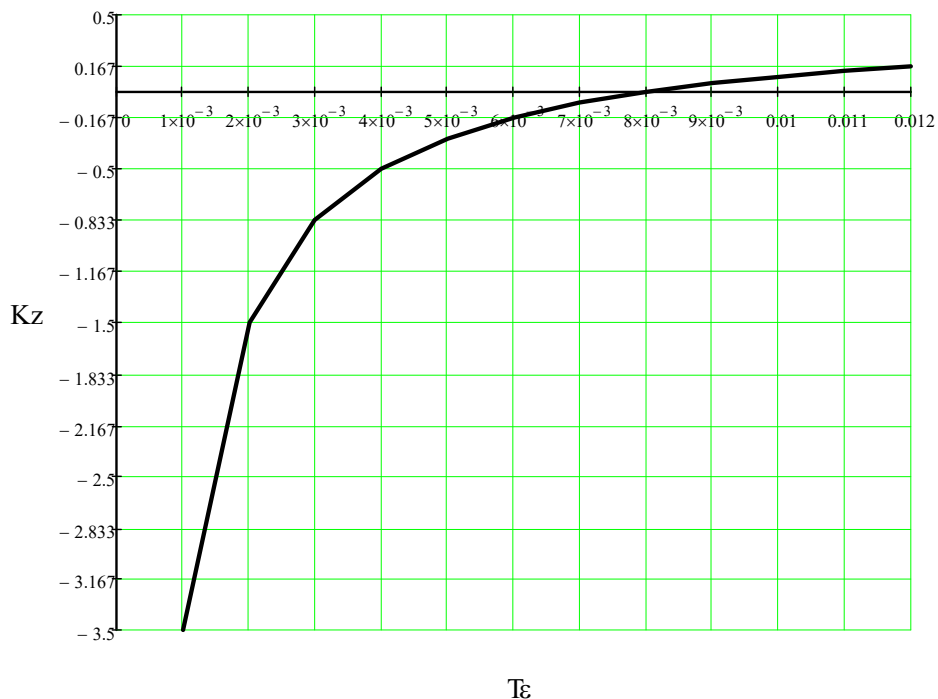
Fig. 4. Dependence of the accuracy margin coefficient on the tolerance capability of the controlled parameter \epsilon . Part material - HVG, processing modes: M=40 , D=8 mm. Spread of technological parameters-10%.
