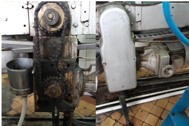
Fig. 2. General view of the conveyor drives: a - with gear; b - with a variator.
