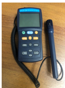
Fig. 3. Appearance and technical characteristics of the PCE-GA 70 combined indoor air quality assessment instrument.
