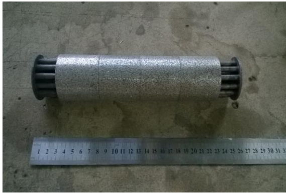
Fig. 1. Porous aluminum inserts.
