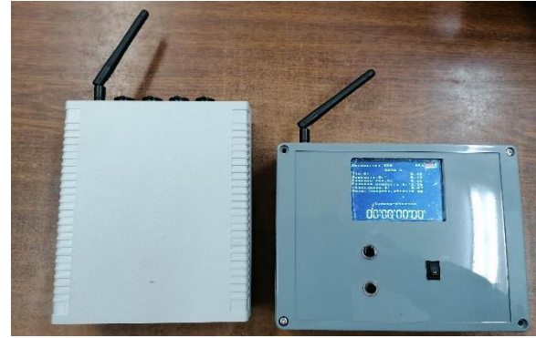
Fig. 2. Appearance of the sensor and the central unit of PTEM -3-W.
