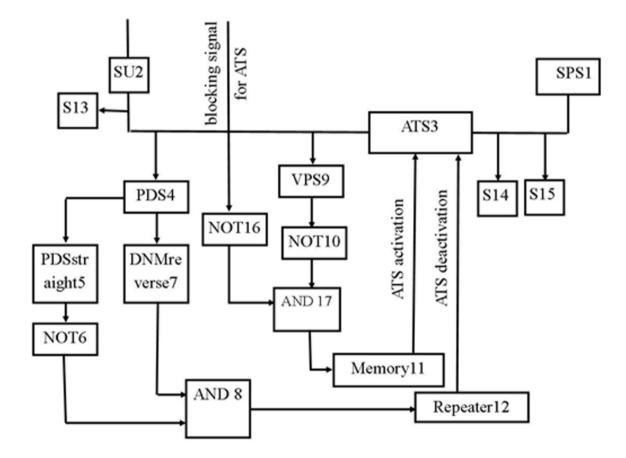
Fig. 2. Structural diagram of a device that implements the method of automatic ATS deactivation.
