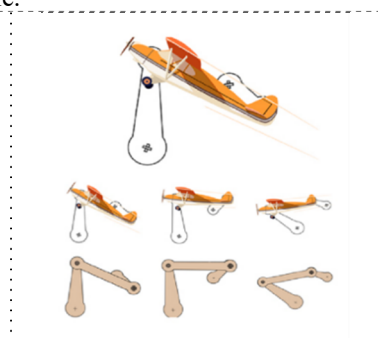
Figure 4. The combination of crank and rocker mechanism and aircraft.
