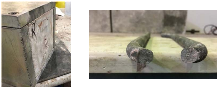
Fig. 7. Test 3- Sheared surface of 16 mm rock bolt in a confined concrete
