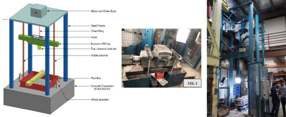
Fig. 2. Drop hammer test and MK-I set up
