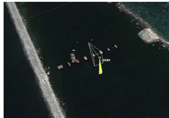
Fig.1 Fixed point acoustic monitoring scheme before the interceptor in an open water channel in the Taishan Nuclear Power Plant
