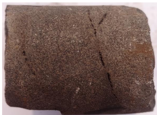
Fig. 7 Fractures in borehole core of Shaximiao sandstone
