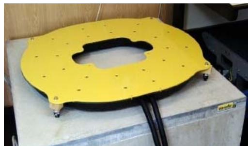
Fig. 7. Disc structure coupling transformer
