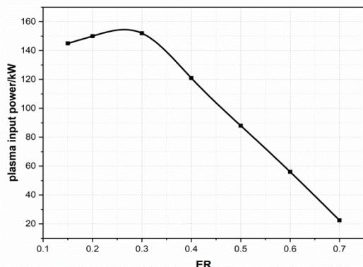
Fig. 3. Plasma input power varying with ER value
