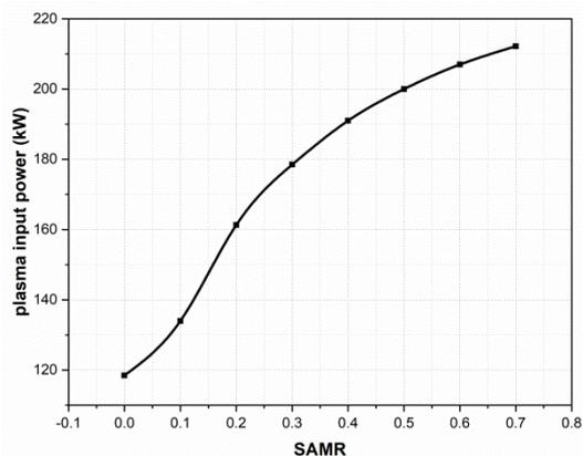
**Fig. 6.** Plasma input power varying with SAMR value
