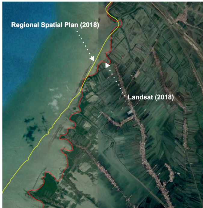
Fig. 10. Coastline change in 2018 according to Regional Spatial Plan and analysis from Landsat Imaging.
