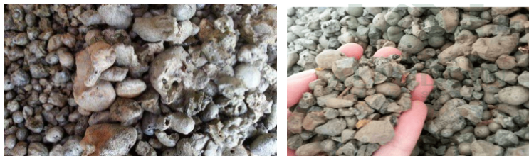
Fig 2. Physical Form of Nickel Slag Waste with Granulation Pond System
