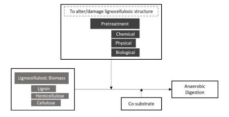
Figure 1. Steps involved to produce biogas from lignocellulosic biomass
