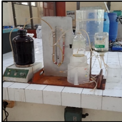
Figure 1. BMP test analyzer
