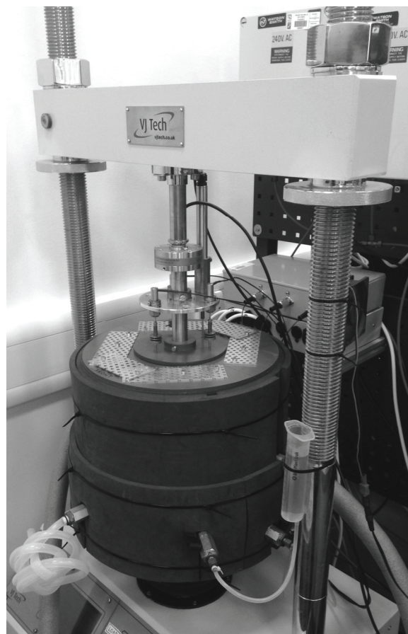
Fig. 2. Temperature-controlled oedometer photograph
