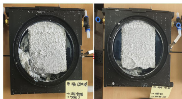
Figure 7. Individual circulation type Mg-Air battery loaded with by-product.
