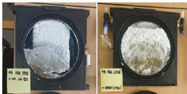
Figure 6. Total circulation type Mg-Air battery loaded with by-product. The left is the state of equation (8) and the right is the state of equation (9)
