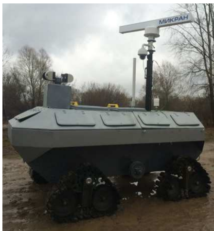
Fig. 1. Mobile robotic complexes with the caterpillar-modular mover
