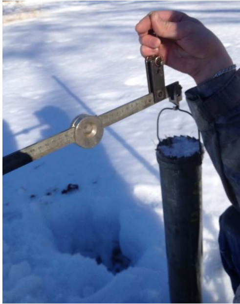
Fig. 6. Weighing the measured volume of snow using the VS-43 device.
