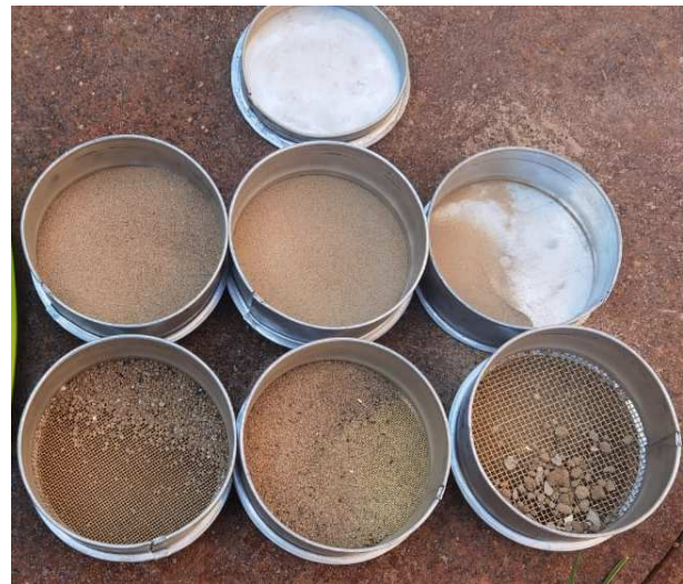
Fig. 5. Sifting sand through sieves of different sizes.
