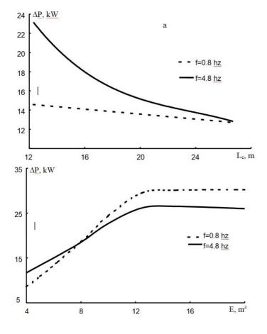
Figure 1. Power loss in the hoist gearbox depending on: a – boom length, b – bucket capacity
