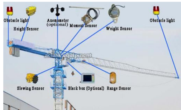
Fig. 5. Safety devices used in tower cranes according to Standards [42]
