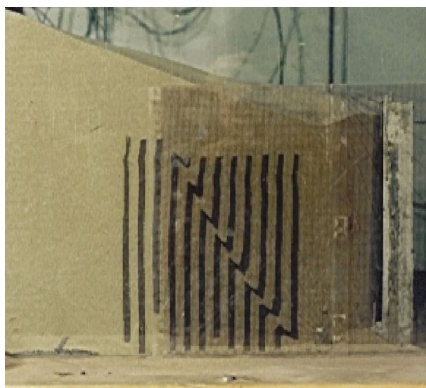
Fig. 3. Slip failure behind the wall [10].
