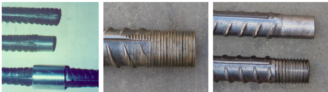
Fig 1. Three Kinds of Straight Thread Joint
